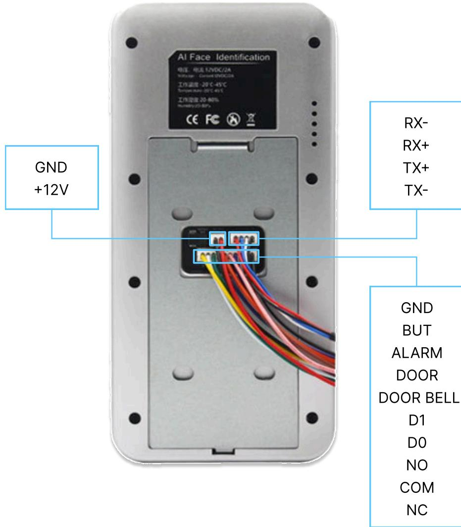
Note: Cable and interface definitions (interfaces may vary slightly between production batches)
